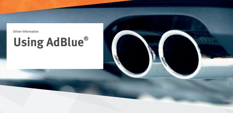
As part of the overall drive to reduce emissions, and to comply with the new Euro 6 standards, more and more diesel cars now include SCR (Selective Catalytic Reduction) technology. Used in the right way, SCR can help to reduce Nitrogen Oxide (NOx) emissions by as much as 90%, with fuel efficiency also increasing by between 3% and 5%.
